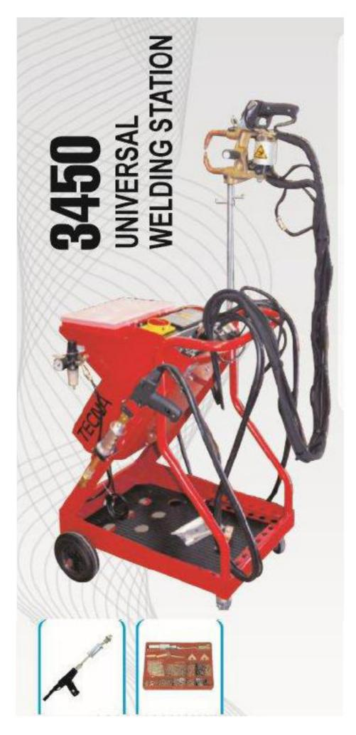
Supply Voltage \*400 V Mains Frequency \*50/60 Hz Mains Protection 25 A (Delayed) Nominal Power50% ED 10 kVA Maximum Welding 50 kVA Power Maximum Secondary 8 kA Current Thermal Current 100% 8 V Weld time 1- 99 Cycles Protection Rating 21 IP Weight 105 kg
